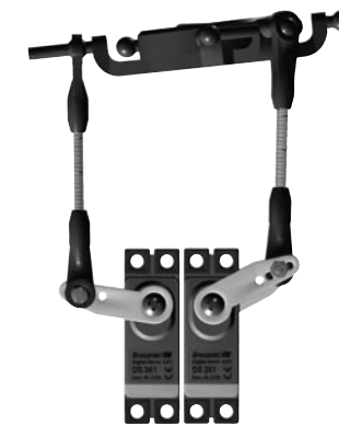
Increase servo travel of elevator servo on one side
