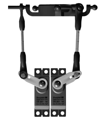
All servos travel the same distance at maximum deflection
