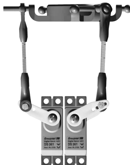
All servos travel the same distance at maximum deflection
