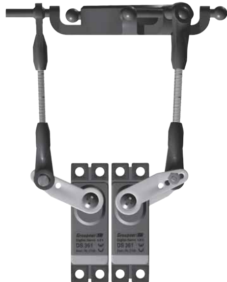
All servos travel the same distance at maximum deflection
