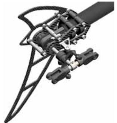
CFK Heckrohr #2758
