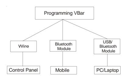
Every Mini VBar unit comes with a USB cable and software which allows for programming it via a PC or laptop. You can also use a mobile phone, blue-tooth module (Mikado item no. 4056) or the special VBar control panel (Mikado item no. 4152). You can switch among these options at any time, so you can program your Mini VBar at home, at the flying field, or anywhere you choose.
