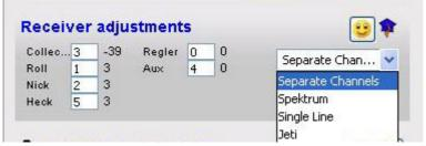
Here you select the applicable receiver. For Spektrum the default is set for DX7, so that the correct channels are automatically assigned. To finish, click on "prepare binding."
