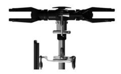
3) It is necessary to install a swashplate driver. Mikado offers a swashplate driver for 10 mm main rotor shafts. It has eight ball bearings: item no. 4018
