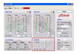
Autotrim is activated in your VBar software by checking the appropriate box. At the flight line, turn on your heli with the collective stick at full positive. Use throttle hold to prevent the motor from starting, until you are ready to fly. Wait until you see a double twitch. The first twitch confirms successful initialization; the second acknowledges activation of the Autotrim mode.
