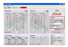
To activate bank switching, choose Bank Selection Bank 0/1/2/3 in the Mini VBar software. Please do not forget to copy your current setup to all the other banks so you have a basic setup on all of them. The status bar "AUX" in the "live display" shows the currently active bank.
