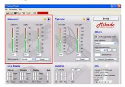
First lets look at the bar "Agility". This bar adjusts the maximum agility of the heli on both the elevator and aileron axis. If your heli reacts to fast, reduce the value. If your heli reacts to sluggishly, increase the value.
