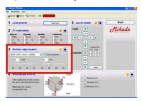
In Step 3 of the setup procedure you can carry out the necessary tail adjustments for the tail assembly. This includes choosing the correct servo type. If your specific servo is not listed, please contact our support team on the online VBar site (www.vstabi.de) to obtain the appropriate setting.
