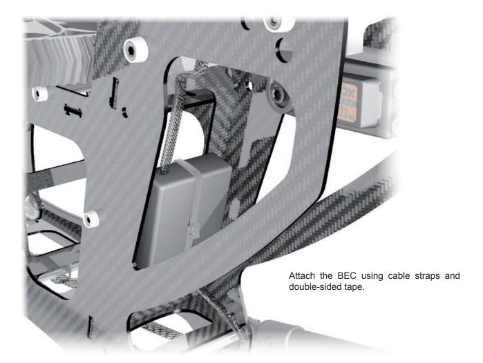
Take special care when placing the wires. Check that the wires cannot rub against the sharp edges of the chassis even if the helicopter should vibrate violently. We recommend to use the fabric tube included here, to protect the wires in suitable places. You may order additional fabric tube (Mikado item no. 4594)
