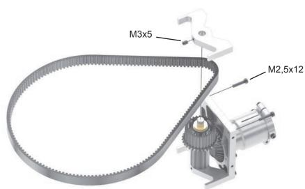
The mainframe of the LOGO 700 XXtreme is pre-assembled. You will find it in Box 1. Note that the screws are not secured. You must use Loctite to secure all screws in the mainframe.
