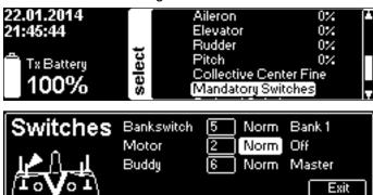
**Optional switches** lets you assign **Option 1-3** functions to switches according to your liking. Later you will assign **Option 1-3** functions within additional apps. For this, you may require additional hardware and/or software.
