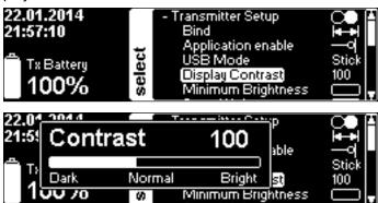
**Minimum Brightness** sets the low threshold for the ambient light sensor. The display will not go darker than the value set here. To save on battery life, use the lowest convenient value.
