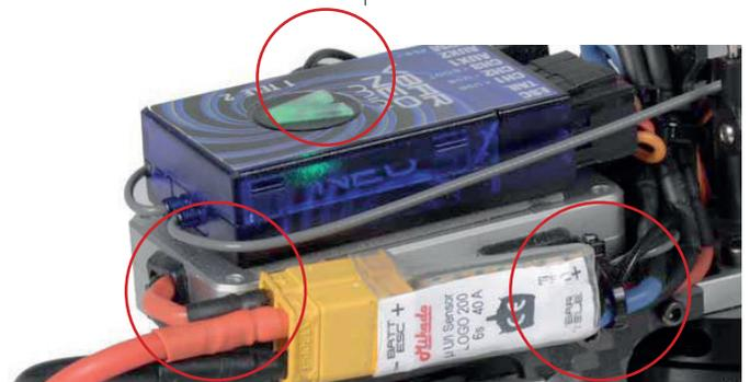
Mounting example LOGO 200: secure with ESC wire and zip tie to motor wires, route sensor wire around ESC/NEO, connect to TELE 1 or 2.
