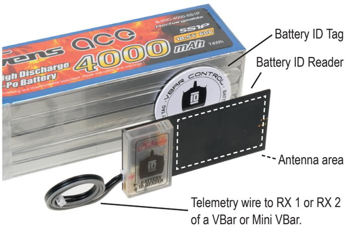
Connect the reader to a VBar (RX 1 or RX 2) using the 3-leaded wire provided. The reader has a second connector where you can daisy chain further VBar Control sensors. The second connector can be left free if it is not needed.
