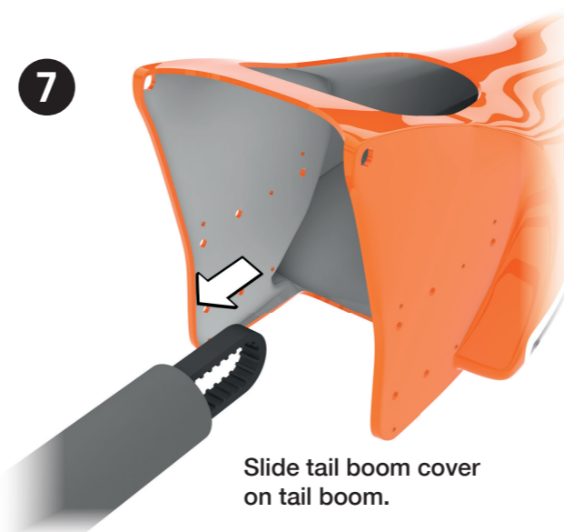
Rearrange wires of tail servo, gyro etc. in a way so they do not touch the tail boom cover. Cut a small groove so the anti static wire does not get jammed between chassis and tail boom cover.
