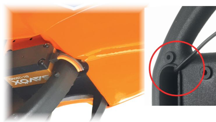
Rearrange wires of tail servo, gyro etc. in a way so they do not touch the tail boom cover. Cut a small groove so the anti static wire does not get jammed between chassis and tail boom cover.
