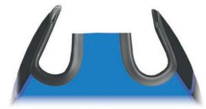
If you want to use the included edge protector, you have to enlarge the cutouts, for a perfect fit. Do a couple of small iterations and check in between, until the canopy sits tightly and braceless. Only then glue the edge protector.
