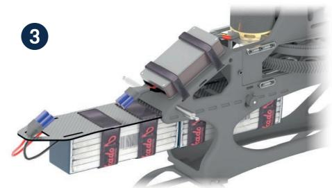
In case the battery plate can only be inserted into the chassis with difficulty in the beginning, please apply a small amount of silicone oil at the edges.
