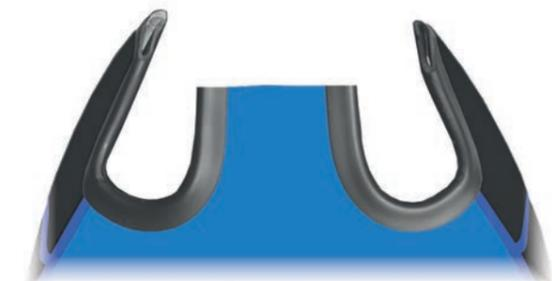
If you want to use the included edge protector, you have to enlarge the cut-outs, for a perfect fit. Do a couple of small iterations and check in between, until the canopy sits tightly and braceless. Only then glue the edge protector.
