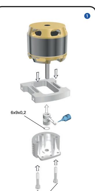
Please mount the motor, motor plate, pinion and counterbearing as illustrated in the above picture. When positioning the pinion, please ensure that it sits exactly on the ball bearing of the counterbearing with only one shim (6.9x0.2) inbetween. Also make sure that the M4 set screw sits on the flattened area of the motor shaft.
