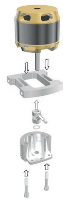
You should position the motor pinion on the motor shaft, before you mount the motor plate. You may also mount the motor pinion at a later stage, but the process will be more cumbersome. For reading on how to mount the motor pinion, please flip to page 9.
