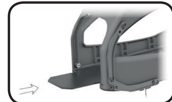
Before you combine the two sides of the main frame, attach the two belt tensioners (#4089, bag 6).
