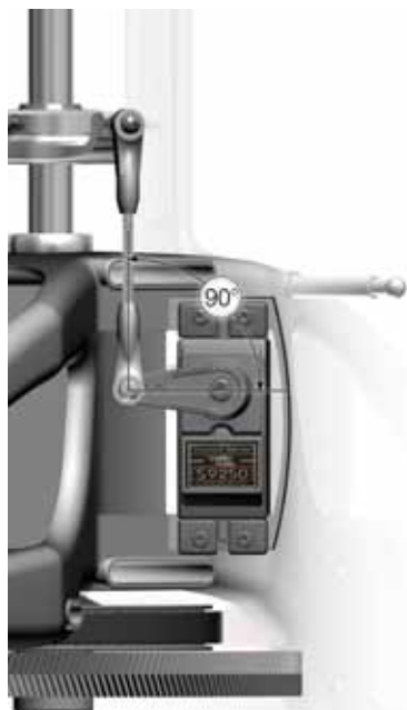
Position of servo arms for the aileron servos when sticks are centered (0 deg. Pitch)
