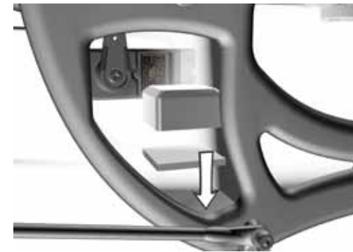
Position for mounting V-Bar gyro
