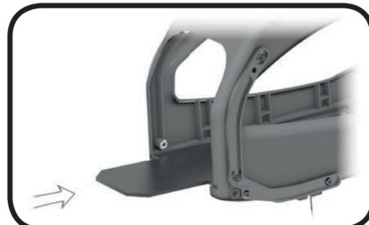
After assembling the chassis, please move the battery plate in to the frame. Should it be hard to move the battery plate please grease the running surface.
