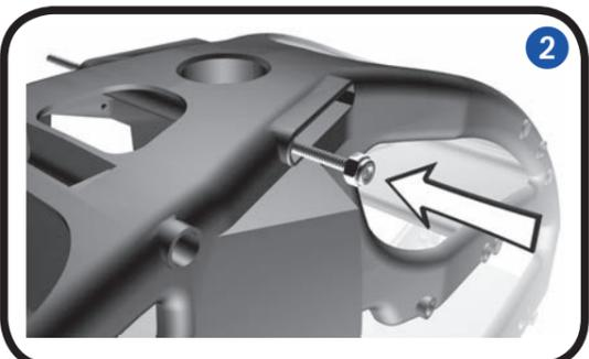
Before you combine the two sides of the main frame, attach the two belt tensioners (#4089, bag 1).
