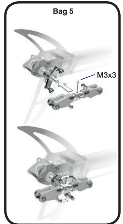
Put a strip of scotch tape on the push rod to avoid wear. Make sure the plastic guide is aligned properly.
