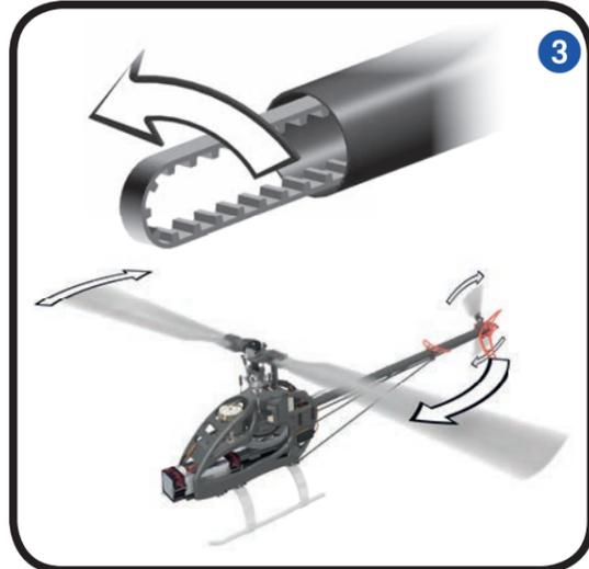
Carefully push in ... Do not damage the tail boom holders and tighten screws.
