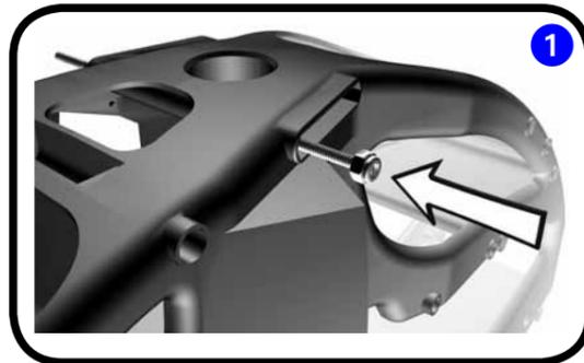
Using the rod M2.5x60 (bag 7), position all 14 nylon nuts in the right side frame.
