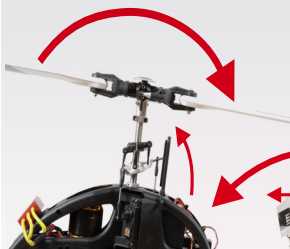
Checking elevator function
