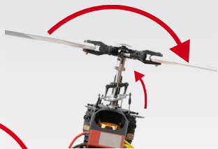
Checking aileron function
