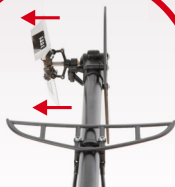
Checking tail function (trailing edges of the tail blades move against the direction of rotation)
